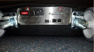
2. Carefully slide the back panel from the simulator until the entire control board can be seen. We will disconnect the wires in 5 steps to simplify the process and ensure that no wires are prone to unnecessary strain.
