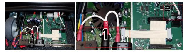
5. The next step is to unplug the audio cables. These wires will be located on the edge of the amplifier board at the top left. You will want to use a jewelers flathead screwdriver to loosen the wires before disconnecting them. After disconnecting, lay these wires to the side next to the power supply wires.
