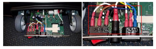
4. After the four power cables have been removed, it is time to unplug the LED power supply located on the right edge of the control board. To do this, just pull to the right and the plug should come out without much resistance.
